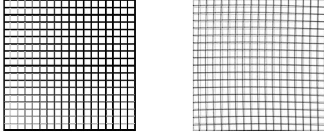
**Fig. 1.** A regular grid (*left*) and a grid subjected to Stirmark attack – small local distortions are visible (*right*)
